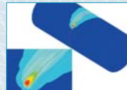
Temperature distribution during the second pass.
