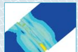
Von Mises stresses in the overlapping area.
