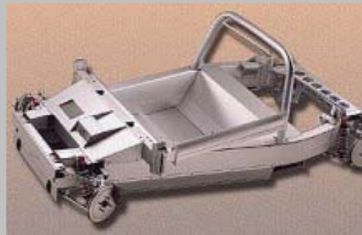
Figure 1: The chassis of the Lotus Elise
