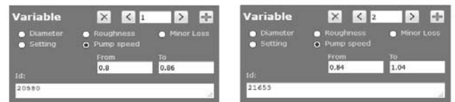
Fig. 10. Selection of pumps for optimization (selection of control variables) and selection of permissible speed ranges.
