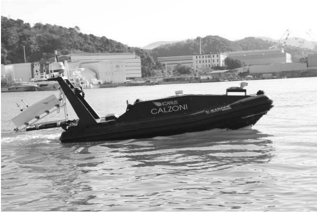
Figure 3: Two Unmanned Maritime Systems (fast mothership carrying a rescue capsule) for search and rescue operations (De Cubber et al. 2013)
